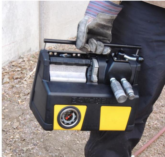
Enerpac XA-12 Air Drive Hydraulic Pump
