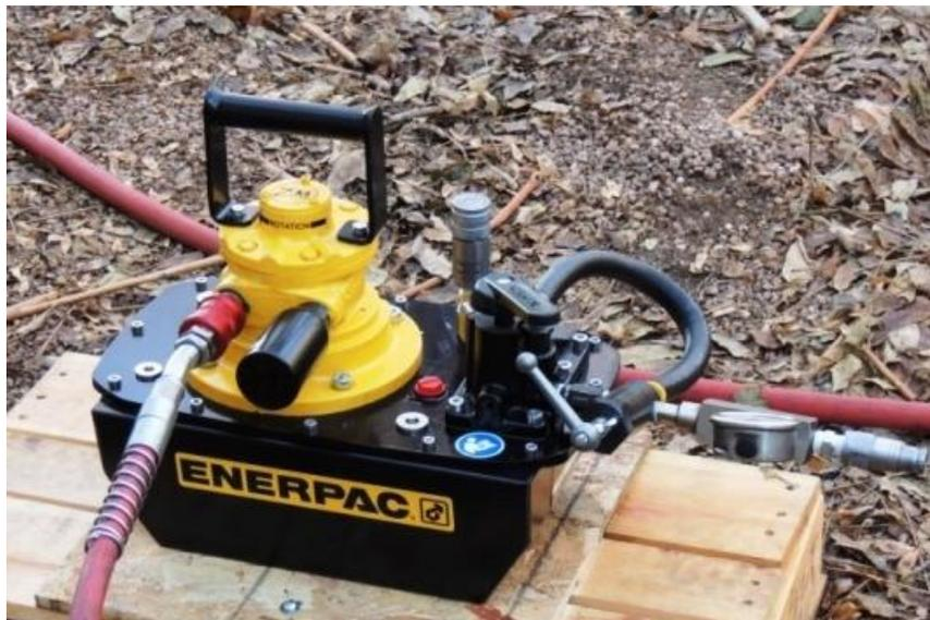
Enerpac ZA-4 Air Drive Hydraulic Pump
